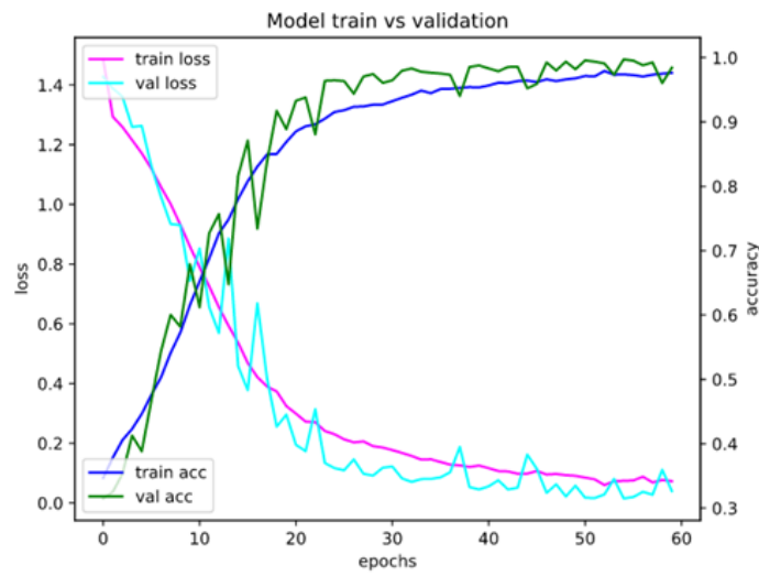
Figure A6. Accuracy and loss on training and test data during classifier training among the set of accents DU, EN, FR, RU .
