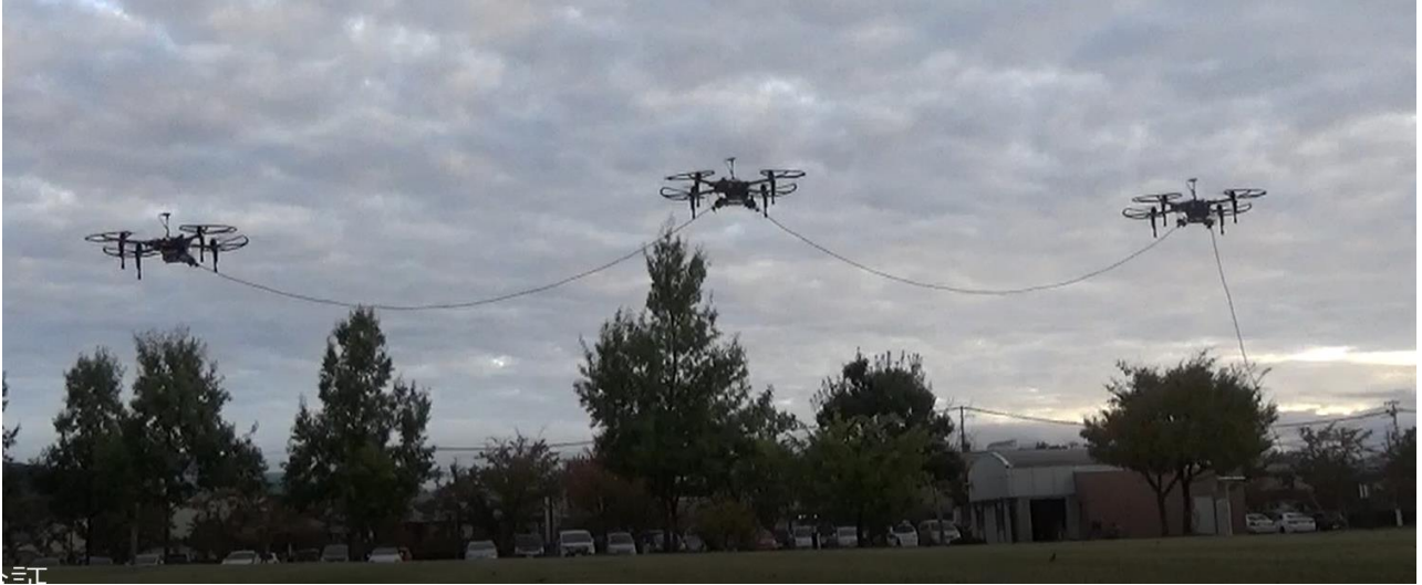
Fig. 9 Flying of a dronet of line connected three drones.
